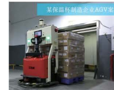
电梯对接 AGV communication with elevator
