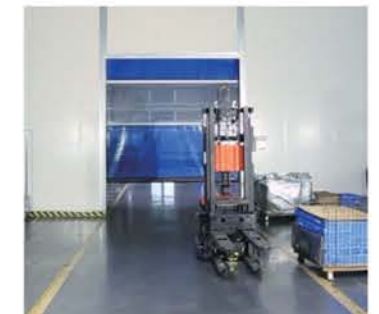
自动门对接 AGV communication with automatic door
